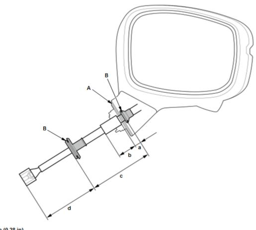
a: 7 mm (0.28 in) b: 60 mm (2.36 in) c: 129 mm (5.08 in) d: 150 mm (5.91 in)
