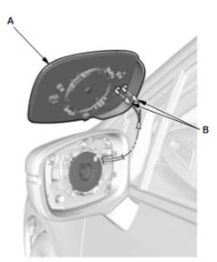
4. With mirror defogger: Disconnect the terminals (B).
